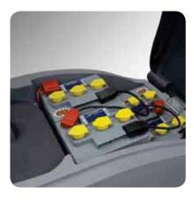
Easy access to battery and vacuum motor compartment, without using tools. Large capacity shock and acid proof polyethilene tanks (88 l) avoid frequent refilling and idle time.  $4 \times 6V$  -180 Ah C5 batteries granting continuous working time up to 4-5 hours.
