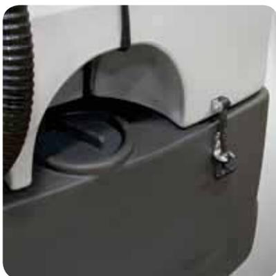
The cleaning solution tank with an exceptional capacity of 300 liters and the high autonomy of the battery ensure a productivity at the top of the range. The wide rear opening allows for an easy and quick refilling of the cleaning solution tank.
