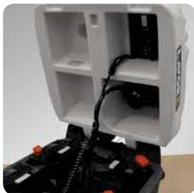
switch with delayed switch-off, brush plate lifting/lowering selector switch, brush motor switch. All motors are protected by thermal breakers. The detergent water tank serves as battery compartment, allowing the housing of great capacity batteries. Battery charger and suction motor are placed the recovery tank; the housing of the
